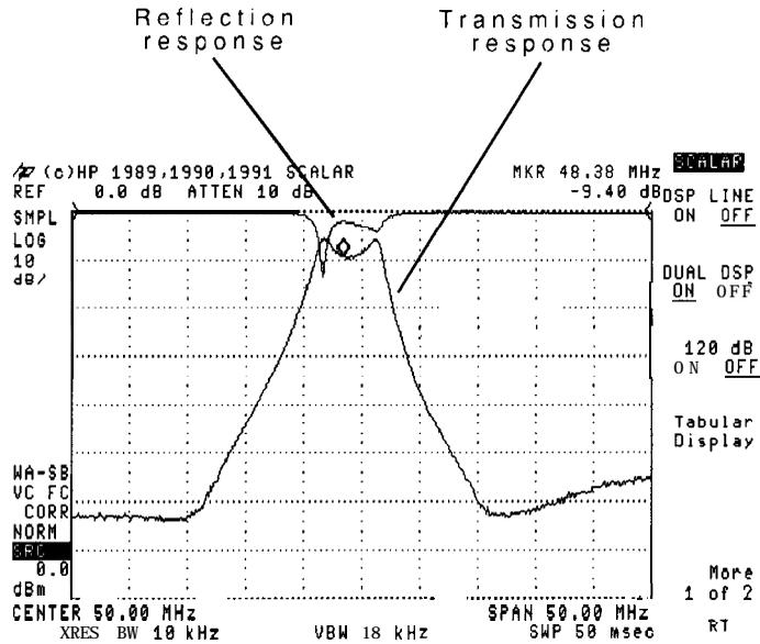
**Step 10. View transmission and reflection results****Simultaneous Results**
