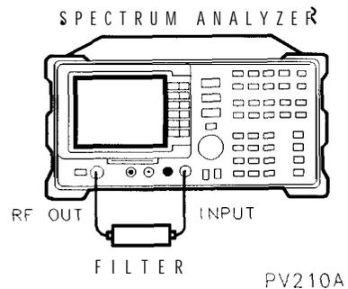
1. Connect the bandpass filter between the input and output.
