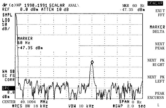
Performing an FFT turns on the marker for locating signal peaks on the FFT.
