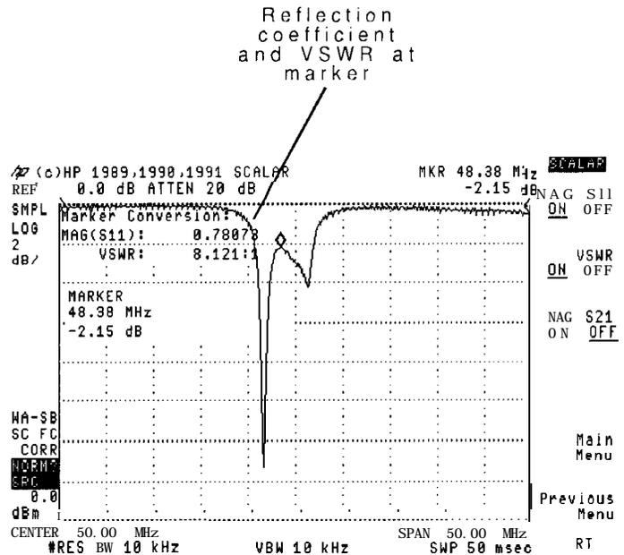
8. Press the **MAG S11** ON OFF softkey so that OFF is underlined.
