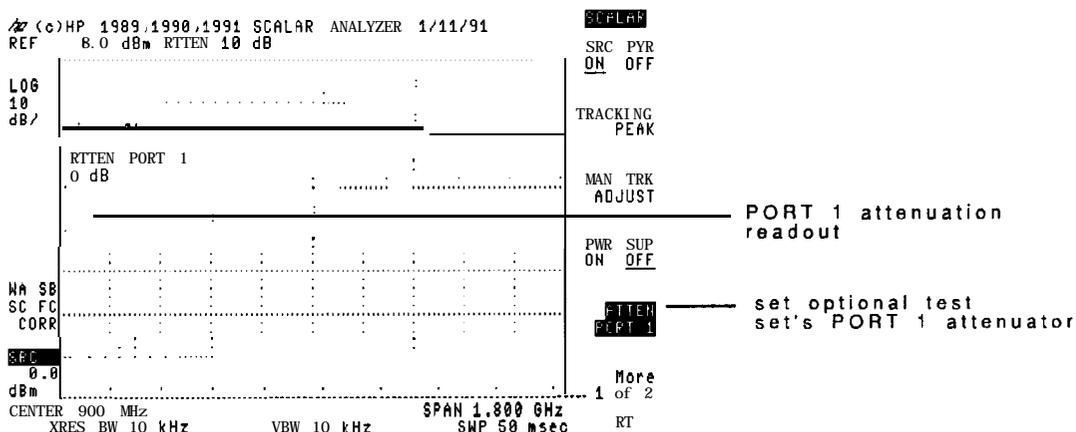
You must inform the scalar analyzer if you have the optional HP 85630A scalar transmission/reflection test set connected. Refer to the following procedure. The scalar analyzer controls the test set through the auxiliary interface on the spectrum analyzer's rear panel.
