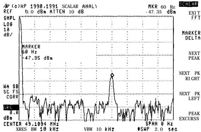
**FFT showing 60 Hz amplitude modulation**
