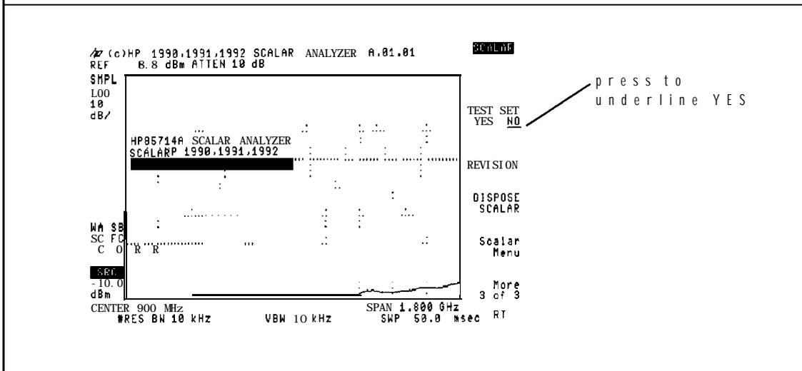
l The scalar measurements personality is now configured for the test set. Turning the spectrum analyzer off or removing the line power does not alter this configuration.
