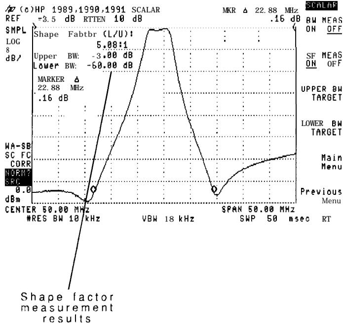
6. Press the SF **MEAS** ON OFF softkey so that OFF is underlined.
