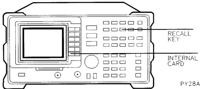
4 Press the following softkeys to load the HP 85714A: CATALOG CARD , **MORE 1 OF 2** , CATALOG DLP ,end LOAD FILE.
