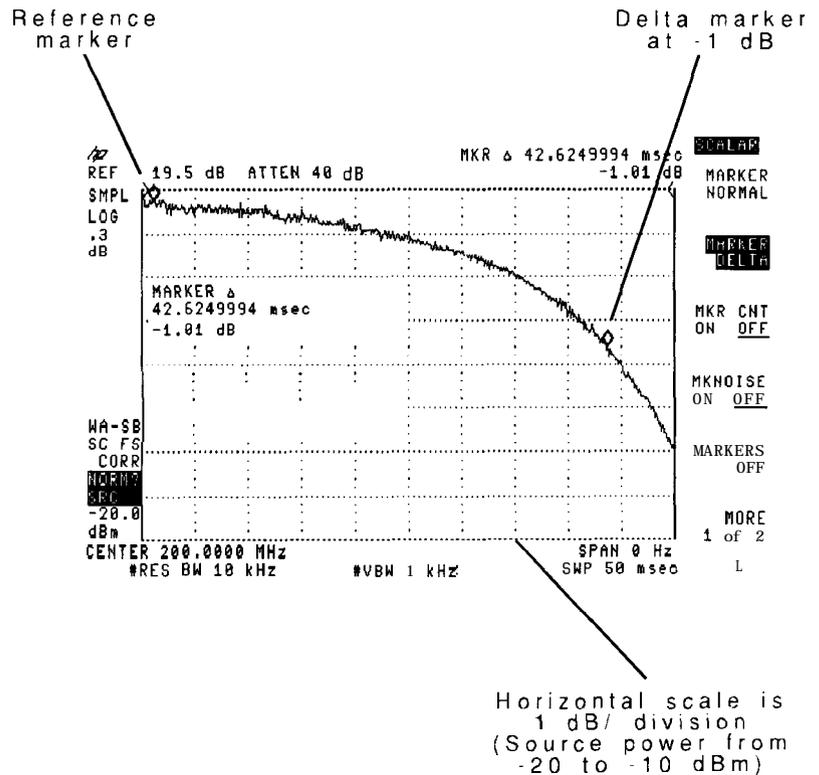
This example measures the 1 dB compression point of an HP 8447A Dual Amplifier. The measurement requires placing the scalar analyzer in a zero frequency span and sweeping the input power to the amplifier.
