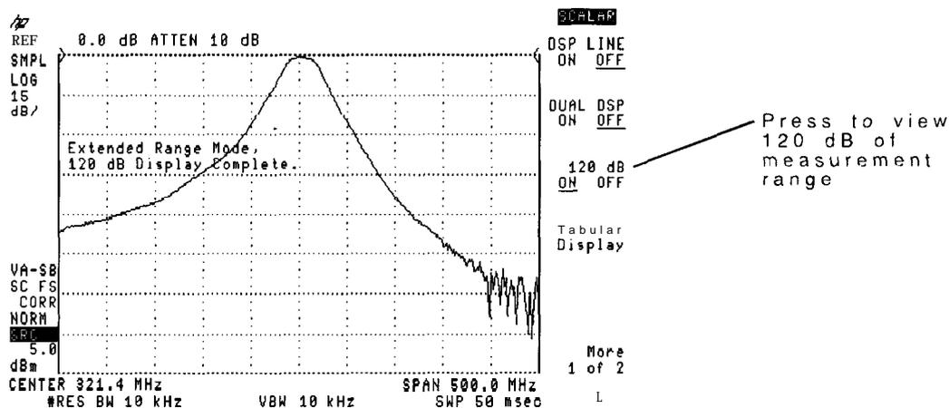
The 120 dB calibrated measurement range is achieved by splicing two separate traces. For each visible sweep, the scalar analyzer first saves the top 50 dB of trace data. Then, the reference level is set up to 50 dB below the current reference level and another reading is taken. Finally, these two traces are spliced together and displayed on the screen.
