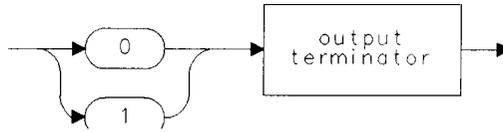
The `ns_DDM` command requires an HP 85630A scalar transmission/reflection test set. This mode is not allowed in conjunction with the extended display range (`ns_EDR`) mode. The default value is off. This command is functionally equivalent to the DUAL DSP ON OFF softkey.
