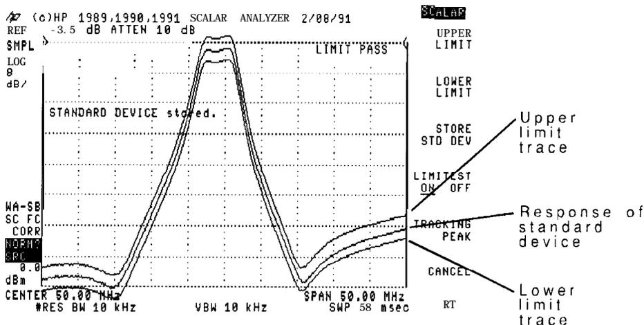
You define the *window* between the upper and lower limit traces using the UPPER LIMIT and LOWER LIMIT softkeys. Enter the amount of deviation in dB between the response of the standard device and the limit trace. The default value is 3 dB.
