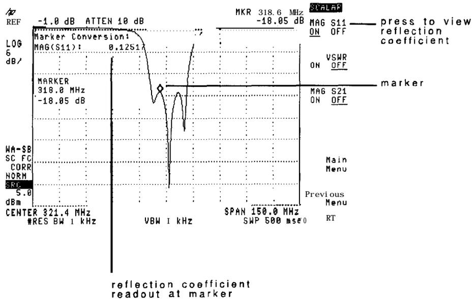
The scalar measurements personality displays a moveable marker showing the value at the marker position. The displayed values are continuously updated. This is true even in single sweep and view modes. Softkeys for these measurements are available from the Measure menu's Marker Convert selection.
