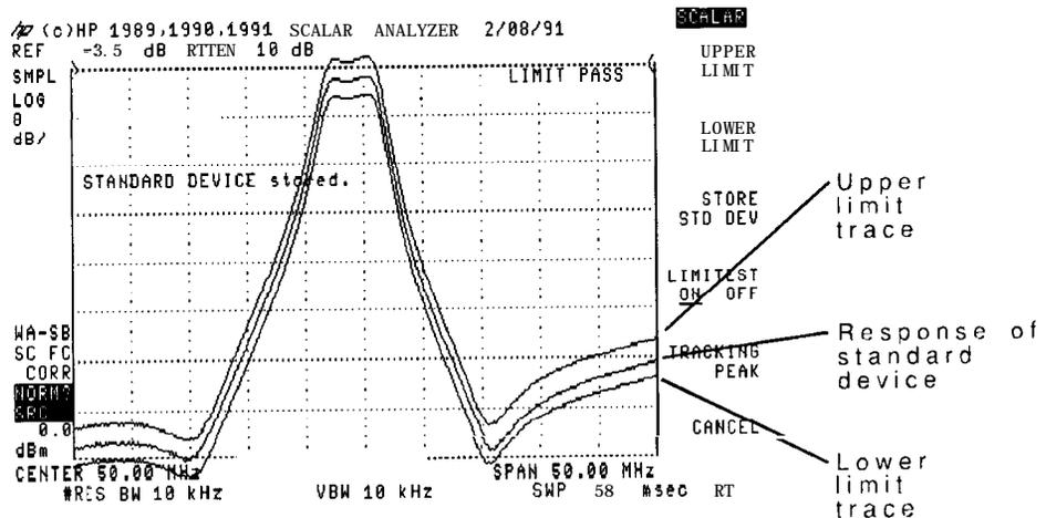
**Step 6. Set up standard device testing**
