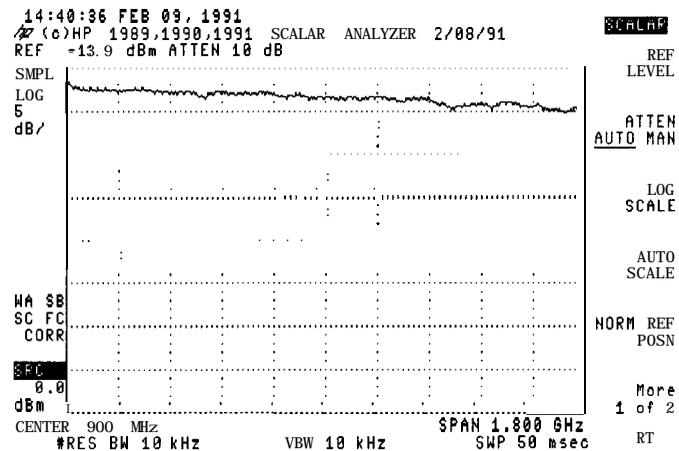
1. Press the **(MKR)** key, and place the marker at the start of the displayed response. This is the start power level.
