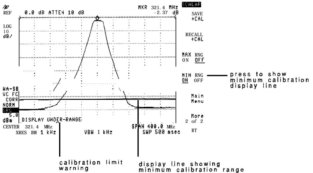
To view the limits of calibration, use the MAX RNG ON OFF and MIN RNG ON OFF softkeys. Horizontal calibration lines are displayed indicating the limits of display calibration. (The lines may not be visible if their amplitude is beyond the displayed scale.) Normally, the calibration lines are turned off.
