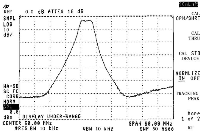
Limit-line testing is turned on (and upper and lower limit traces displayed) after pressing the **CAL** key and then the CAL STD DEVICE softkey.
