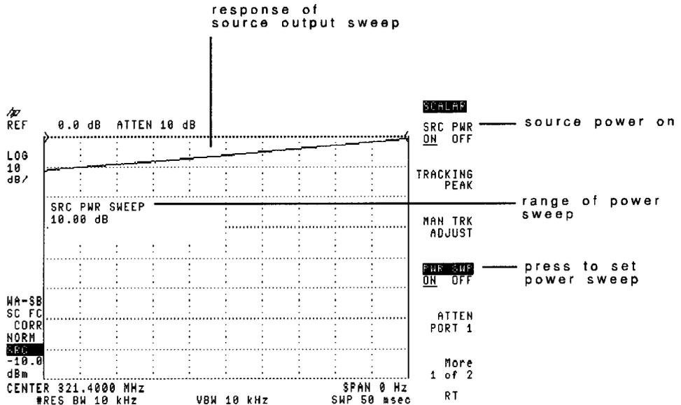
The normalizing capability of the scalar measurements personality enables viewing of the response compression.
