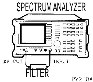
1. Connect a bandpass filter between the input and output.
